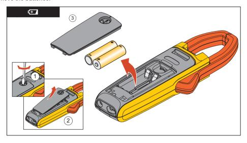
Figure 3. Remove Batteries
