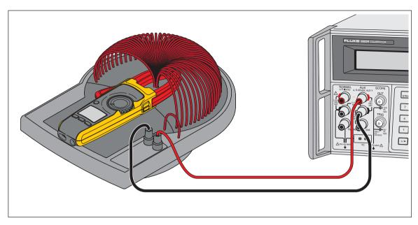
Figure 5. Current Calibration Setup
